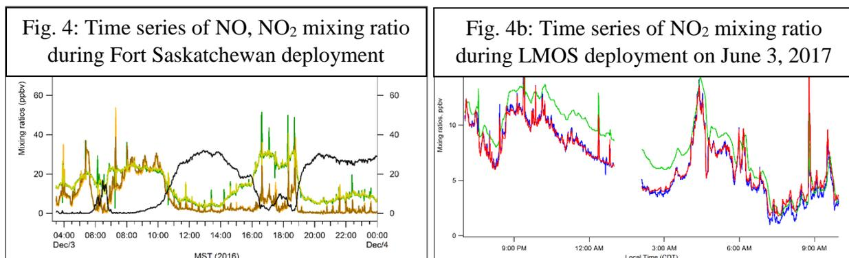
Fig. 4a: (Green): NO<sub>2</sub> measured by PhoNO-Thermo 42i system, (Yellow): NO<sub>2</sub> measured by Thermo 17i, (Brown and Orange): NO measured both instruments respectively, (Black): Ozone. 4b: NO<sub>2</sub> mixing ratios of PhoNO (blue) compared to CAPS (red) and FRM (green) instruments. CAPS and PhoNO match closely while FRM NO<sub>2</sub> reads higher mixing ratios
