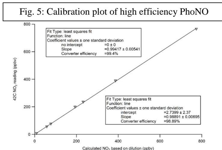
Fig. 5: High efficiency PhoNO calibration plot
