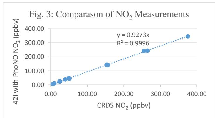
Fig. 3: Shows a calibration of a PhoNO-Thermo42i system with CRDS NO<sub>2</sub> measurement
