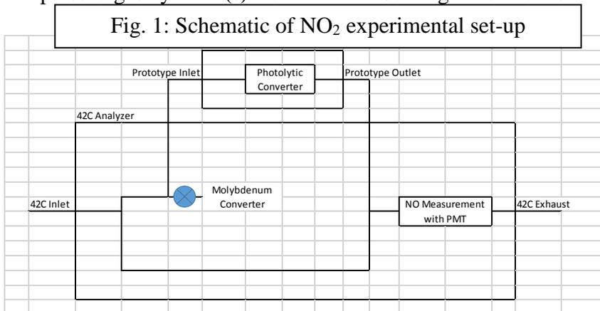
Fig. 1: Schematic of the sample flow through the 42C/42i analyzer and the PhoNO system
