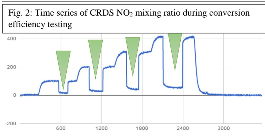
Fig. 2: Shows a time series calibration of a PhoNO-Thermo42i system with CRDS NO<sub>2</sub> measurement. The y-axis is in units of ppbv and x-axis is elapsed time (seconds). Green arrows show when the PhoNO device was turned on prior to NO<sub>2</sub> detection by the CRDS instrument.
